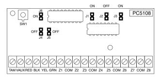
**NOTE:** Only jumpers J1, J2, and J3 determine the zone assignment for the module
